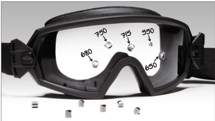
MilSpec goggle standard Requires impact at 550-560 feet per second. Impacted by a 0.22 Caliber 17 Grain, T37 shaped projectile at varying feet per second.
