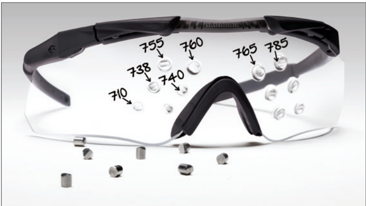
MilSpec spectacle standard Requires impact at 640-660 feet per second. Impacted by a 0.15 Caliber 5.8 Grain, T37 shaped projectile at varying feet per second.
